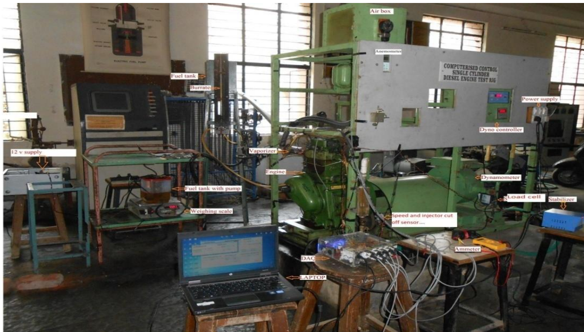
Fig 2.1 Actual experimental set-ups for modified engine (HCCI engine) A vertical, single cylinder, water-cooled, four stroke, and high speed diesel engine has been used for the experiment. The technical specification of engine is as under:
